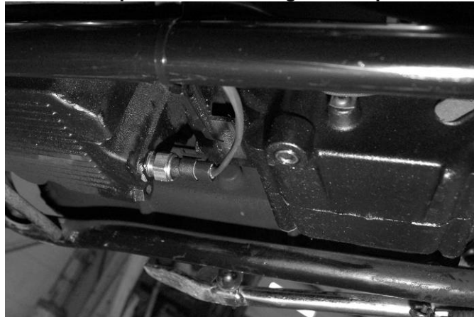
Installed oil temp sensor and harness plug
