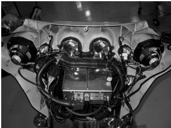
Pic of Street Glide with outer fairing removed
