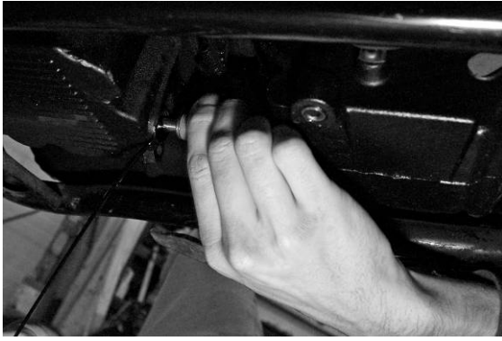
Thread sender into oil pan
