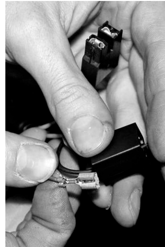
Remove the pin from the connector
