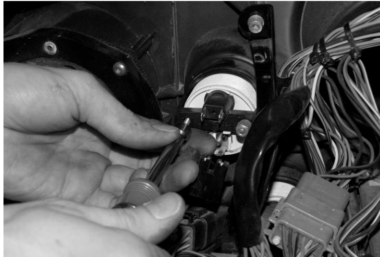
Remove the small gauges with 5/16" wrench or nut driver
