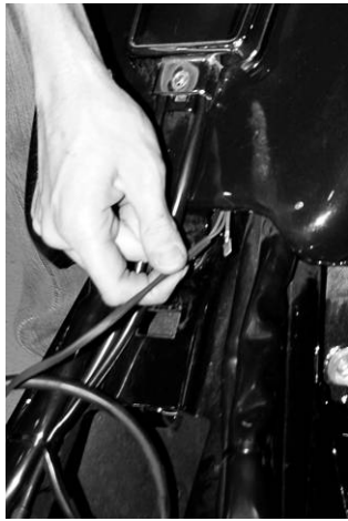
Route wires under tank
