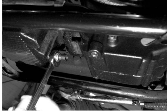
Tighten temp sensor with a 3/4" wrench
