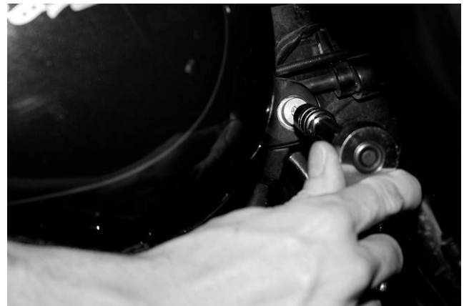
Remove front tank bolts to loosen tank
