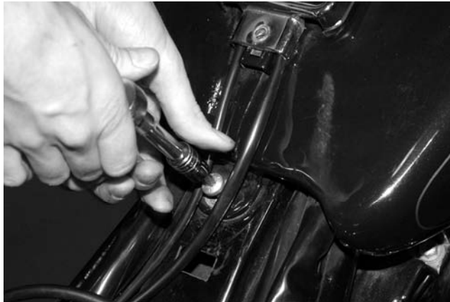
Remove rear tank bolt
