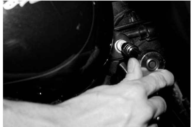
Remove front tank bolts to loosen tank
