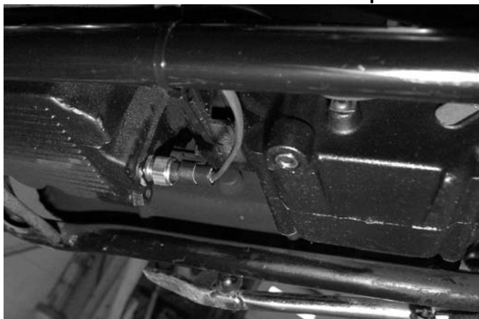
Installed oil temp sensor and harness plug TC
