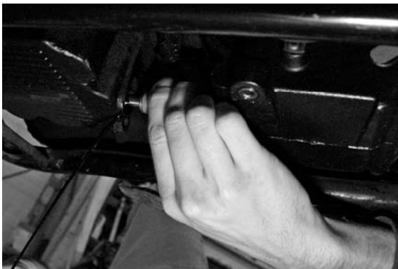
Thread sender into oil pan
