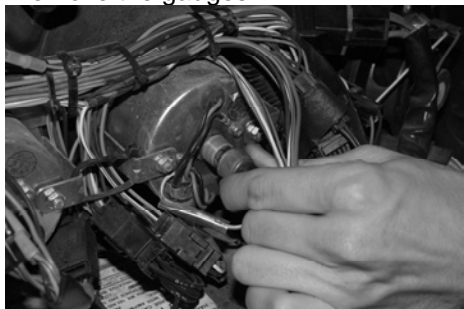
Remove speed cable/unplug gauges
