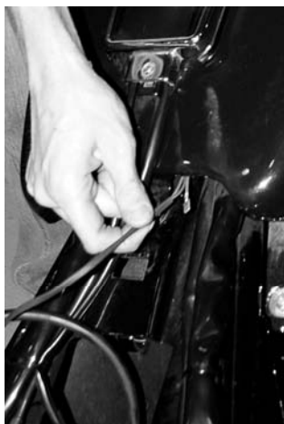
Route wires under tank
