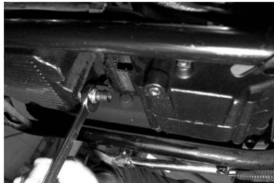
Tighten temp sensor with a 3/4" wrench
