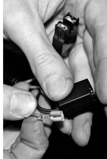
Remove the pin from the connector
