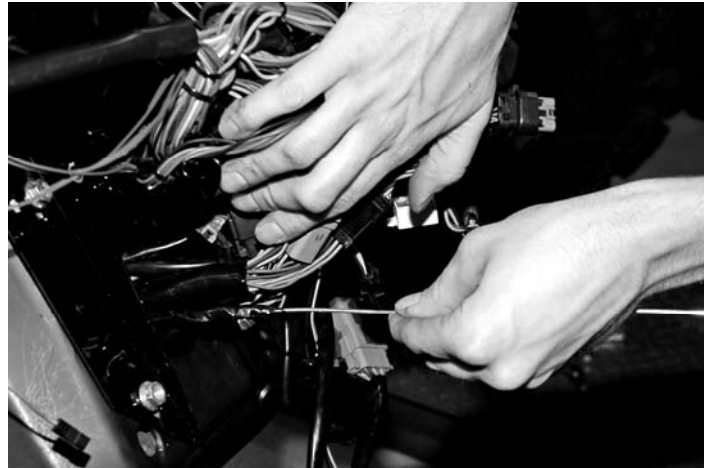
Pull the temp sensor wires through the fairing
