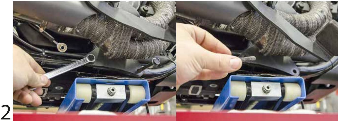
Remove oem right footrest bolt.
