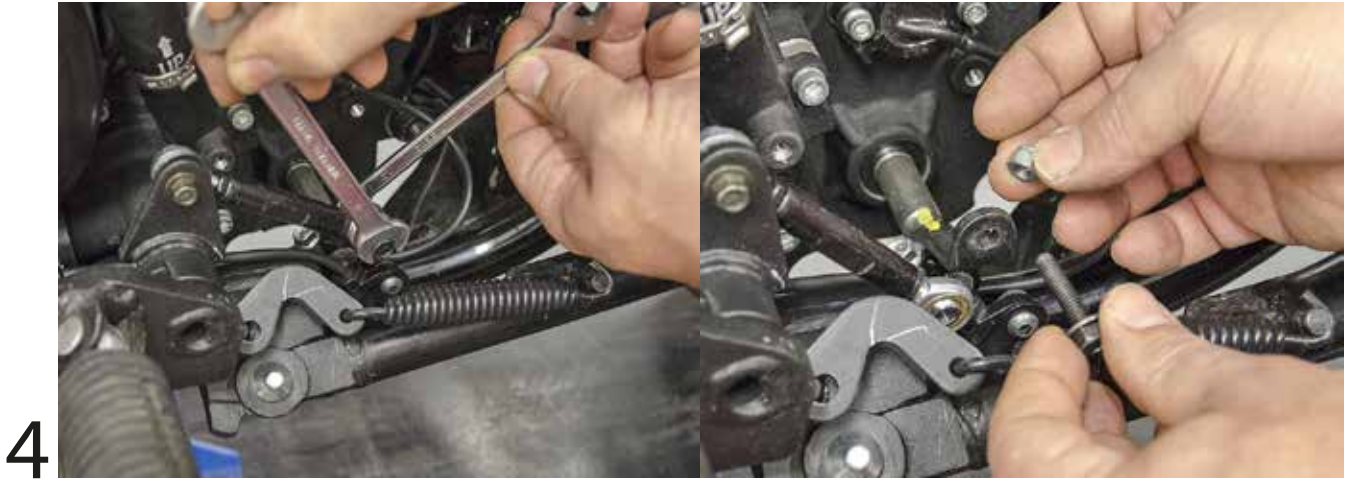
Remove bolt that connects the shifter rod.
