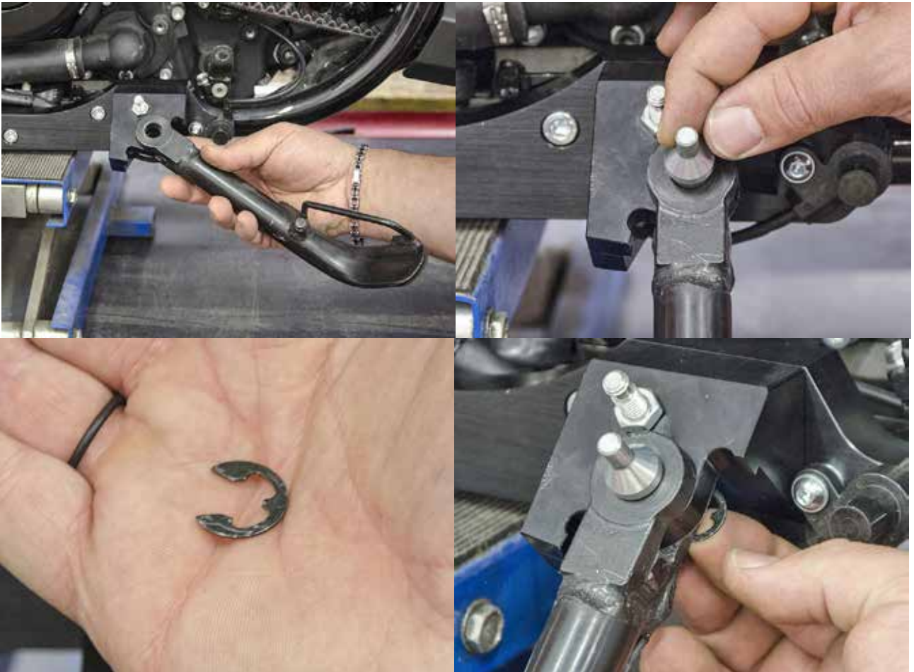
Attach side stand and secure with pin and snap ring oem.
