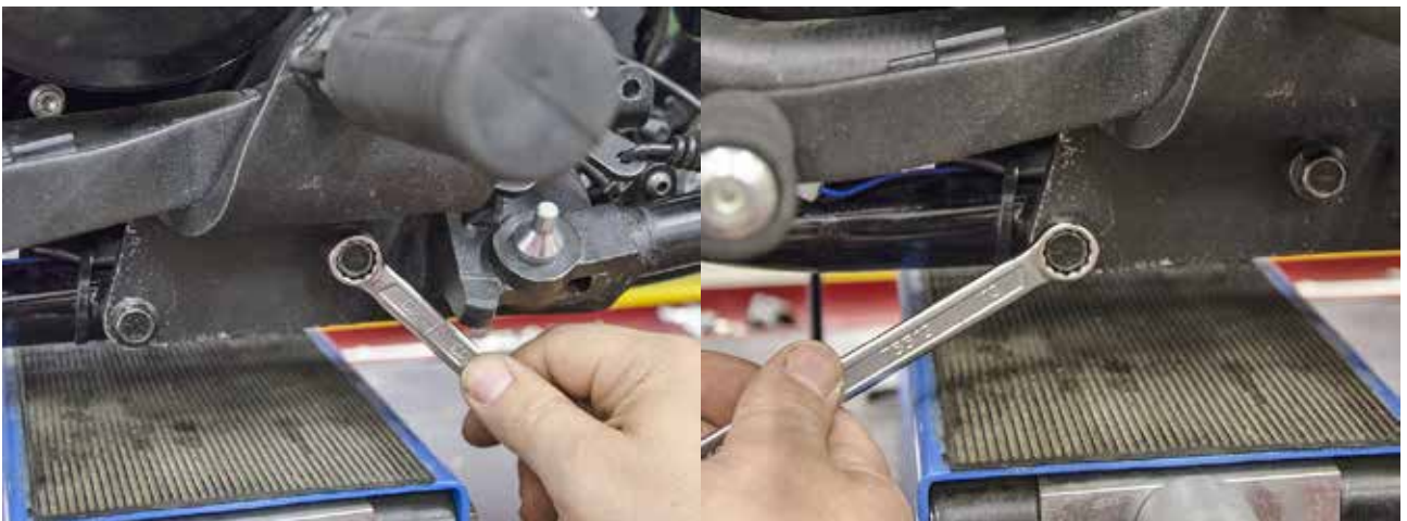
Unscrew two remaining bolts that hold the oem left footrest.
