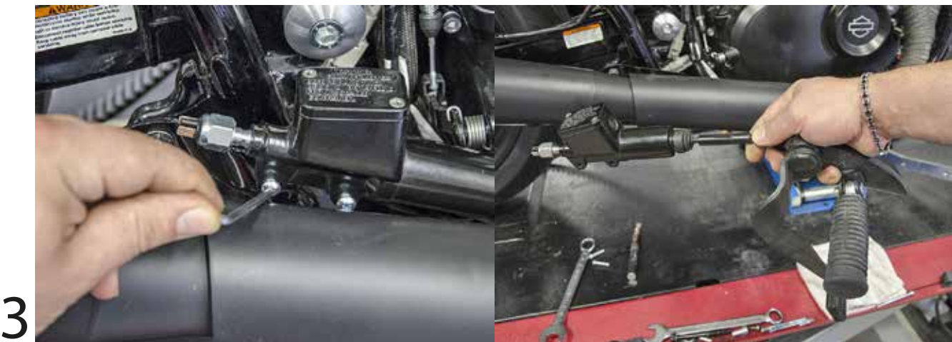
Unscrew the bolts that hold the master cylinder and remove footrest.
