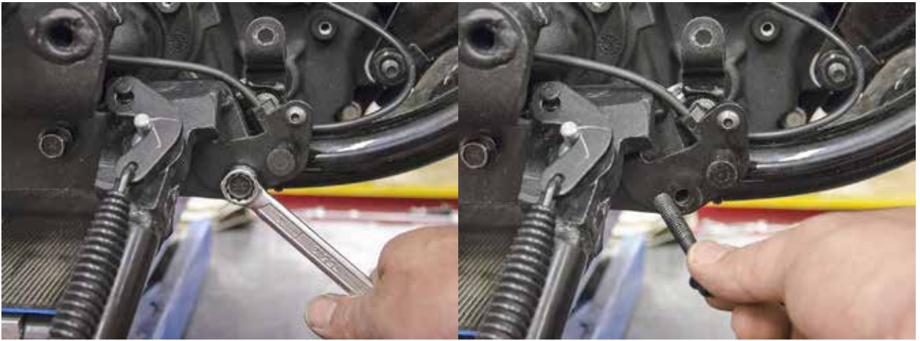
Remove side stand sensor.
