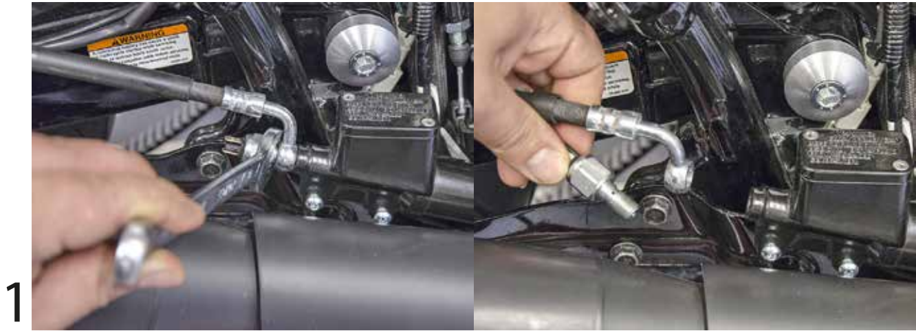
Remove brake light switch and hose.
