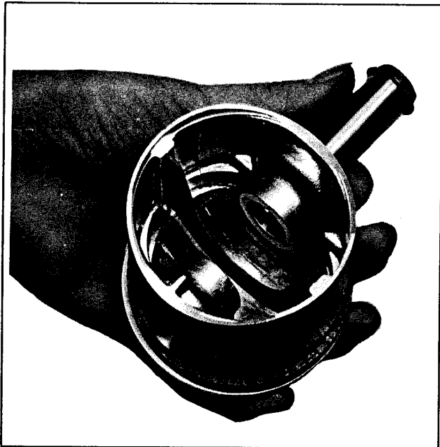
Figure 3C-13. Piston with Web on Right Side
