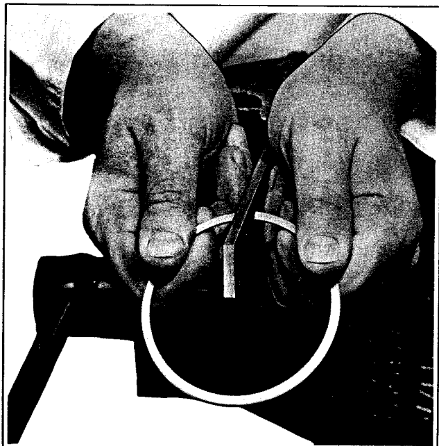
Figure 3C-8. Filing Ring Gap
