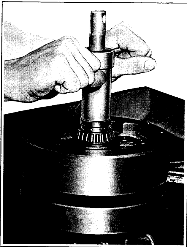
Figure 3E-16. Pressing Bearing on Sprocket Shaft
