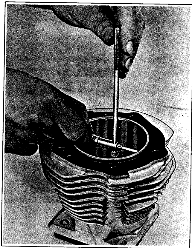
Figure 3C-4. Measuring Cylinder Bore
