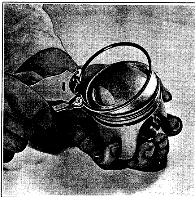
Figure 3C-9. Assembling Rings with Ring Expander
