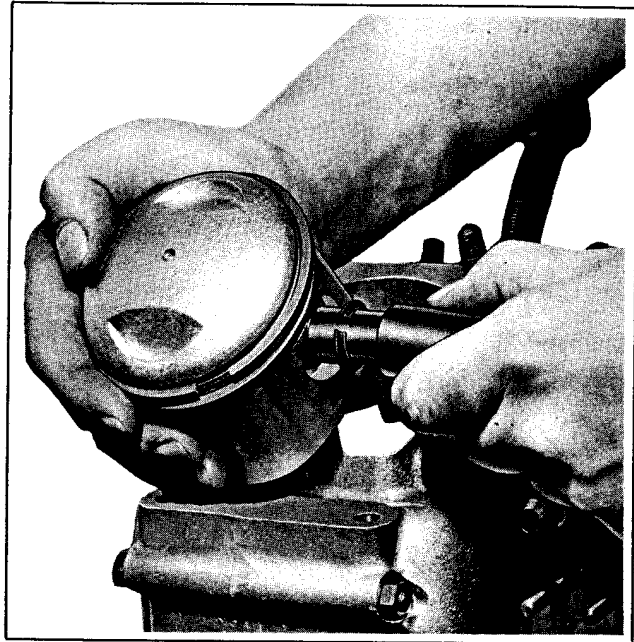
Figure 3C-14. Inserting Piston Pin Lock Ring
