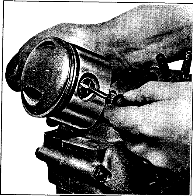
Figure 3C-2. Removing Piston Pin Lock Ring
